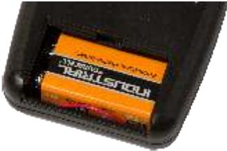
Place the battery into the battery compartment making sure that the battery connector is to the left-hand side (as you look at it) and the battery cable runs along the bottom of the battery compartment.
